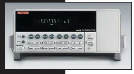
The 5½-digit Model 6485 Picoammeter combines Keithley's expertise in sensitive current measurement instrumentation with enhanced speed and a robust design. With eight current measurement ranges and high speed autoranging, this costeffective instrument can measure currents from 20fA to 20mA, taking measurements at speeds up to 1000 readings per second.
